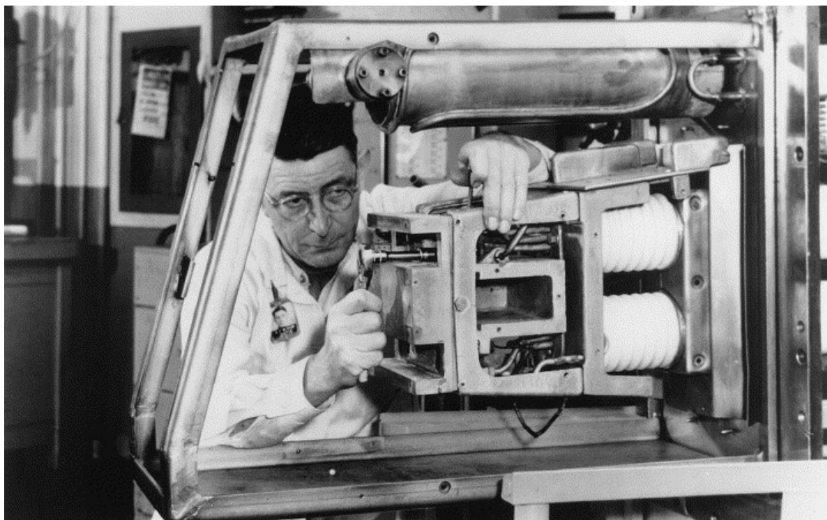
Figure 3.1: One of the beta unit calutron sources. ORNL Photo 24574, from Yergey and Yergey (1997).
